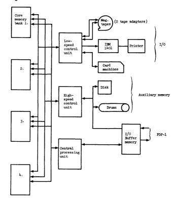
Fig. 1 Characteristics of the AN/FSQ-32 Storage Devices
